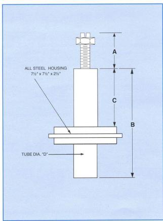
Heavy Duty JAKEBOLTS offer a truly cost effective way to provide strong, problem-free, high quality anchors for virtually any concrete foundation/machinery application. They are designed to be hung from a template or welded directly to reinforcing steel, then cast in place during new foundation contruction.
